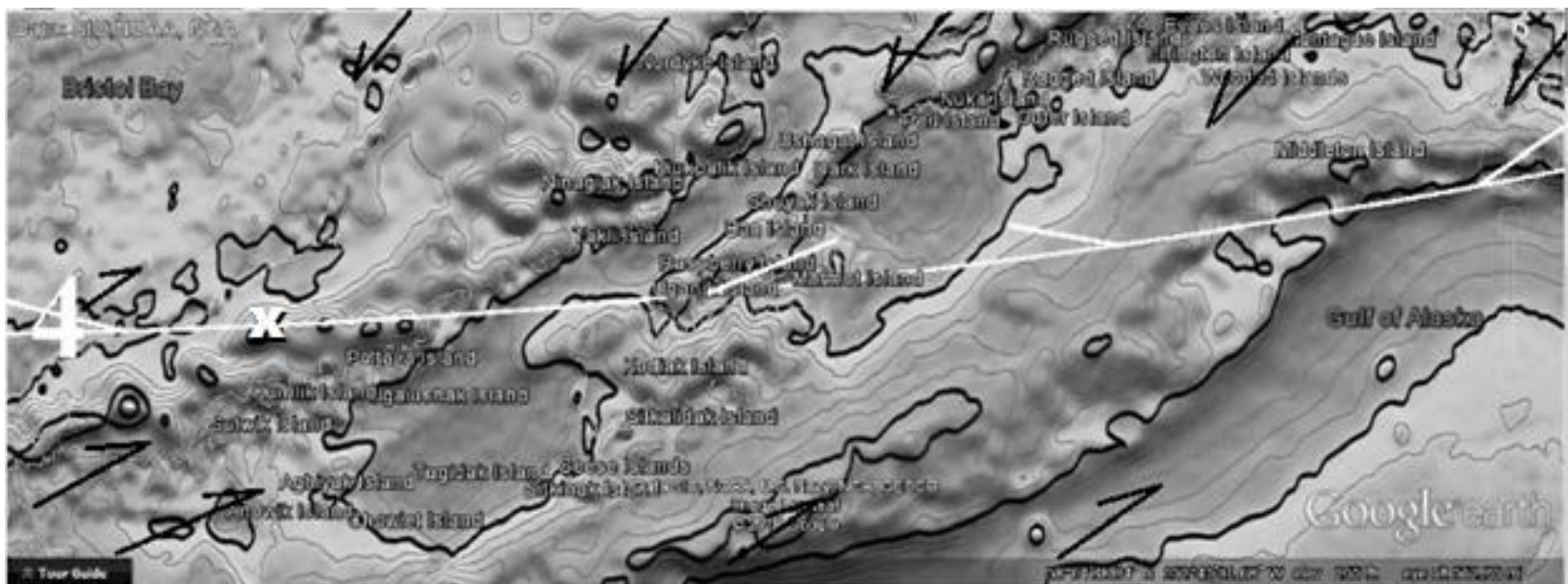
Figure 4.19: Global Gravity Anomaly overlay of CGRS 4 showing two major directions of CGRS causing a complex signature. Five or more obvious arcuate lineaments cross CGRS 4, running NE/SW (black arrows). The shift from elevated to lowered gravity readings suggests interference. Clear changes expressed in both highs and lows can be seen in the linears. X = point on Table I. (Google Earth, accessed 8/20/2016.)
