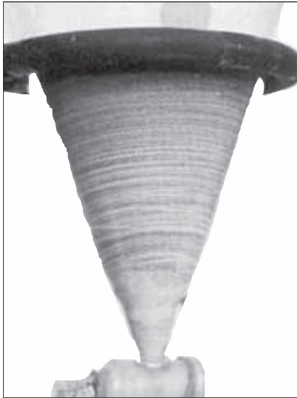
Figure 15. Hyperconcentrated laminar bedforms produced by swirling a wet heterogeneous sediment mixture and drawing the liquid out the bottom. Note large number of “laminar strata” produced atop each other in an instant of time. From Berthault (1988, figure 1).
